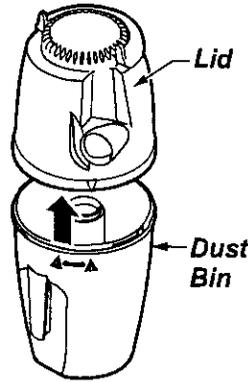
Separate the lid from the dust bin by lifting it straight off.
